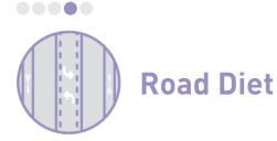
A road diet reduces the number and/or width of travel lanes to allocate space for other facilities such as bike lanes, sidewalks, buffer zones, and/or on-street parking. A road diet can create the perception of a narrow lane width, thus reducing travel speeds.
