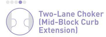
Chokers are curb extensions at midblock that narrow the street. They leave the street cross section with two lanes that are narrower than the normal cross section. Their effectiveness in calming traffic is limited by the absence of vertical or horizontal deflection, but can still be beneficial.
