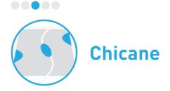
A chicane is a variation of a lateral shift. It includes a series of alternating mid-block curb extensions or islands that narrow the street and require drivers to navigate a curved path, thus reducing vehicle speeds.
