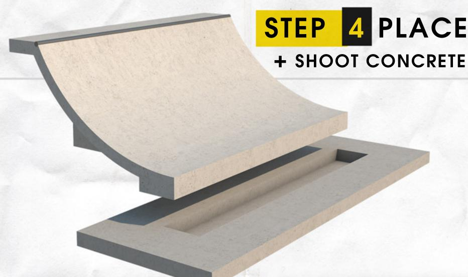
New features and terrain are formed up and rebar is doweled into the existing slab in preparation for placing/shooting concrete. Concrete is finished to the edge of the cutout for a seamless blend with the original slab. Note, elements and terrain that do not transition into the slab (ie. manual pads, ledges, stairs, etc.) do not require cut-outs and are built directly on top of existing concrete.
